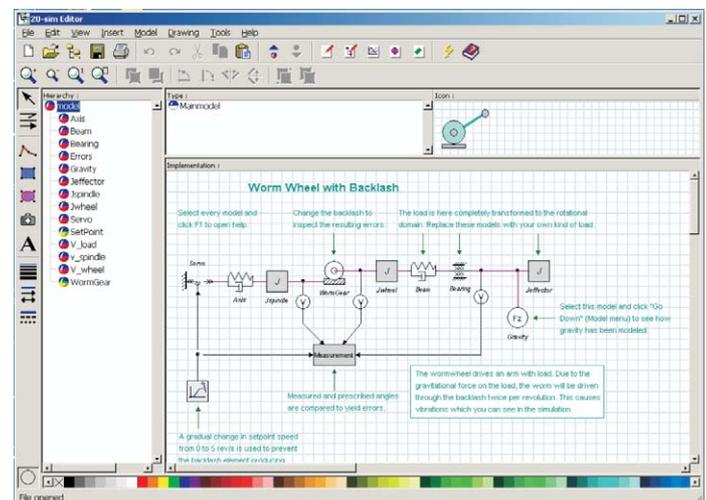
Figure: 3 Worm Gear System model
