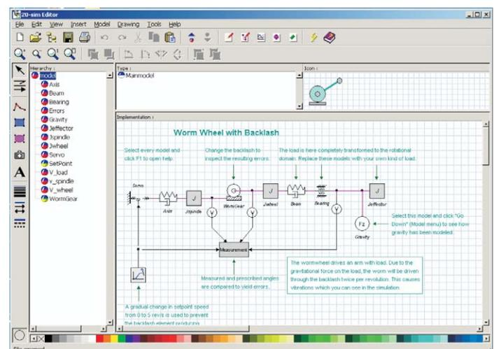
Figure: 3 Worm Gear System model
